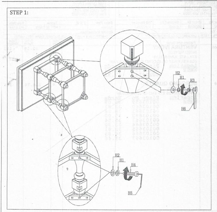
Step 1: Attach Leg (C) to Stretcher panel (B) and Table Top (A) using Flat Washer (H2), Lock Washer (H1), Allen Bolt (H4) by Allen Key (H5) For Stretcher panel (B) and hex nut (H3) by open wrench (H6) For Table Top.
