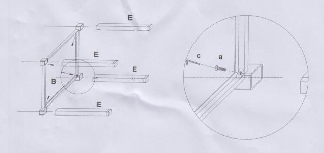
Step2. Assemble the Top Frame(A) to the Acrylic Rod(E)as shown.
