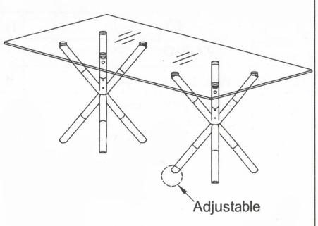
ATTENTION: WHEN YOU ASSEMBLE, PLS DON'T TIGHTEN EACH SCREW UNTIL ALL SCREWS ARE LINED UP WITH THE FRAME.
