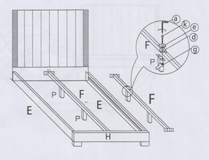
STEP 5 Insert center plastic slot ( i ) into holes on center support bar (F). Press firmly into place as shown in diagram. Attach rail plastic slat ( h ) using same procedure.
