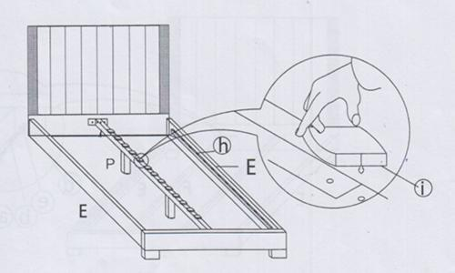
STEP 6 Insert small slat (I) into plastic slats (h, i) as shown in diagram. Attach long slat (L) to Siderail (E) with bolt f as shown.
